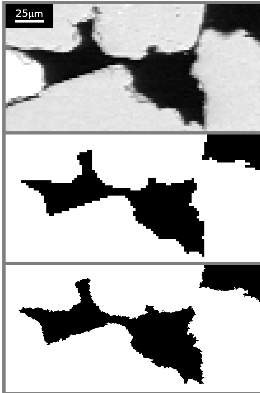
Figure 3.11: Downscaling example, top: extract from coarse scale SEM image at 2.12 \mu\text{m}/\text{pixel} , middle: segmented image, bottom: downsampled image at 0.27 \mu\text{m}/\text{pixel}
