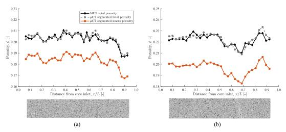
Figure 3: Slice averaged porosities for the two Bentheimer samples calculated using segmented  $\mu$ CT images and differential medical CT images. (a) Core 1, slice width = 1.8mm. (b) Core 2, slice width = 1.9mm. Underneath the porosity graphs is the central slice of the raw, unfiltered dry scan for each core, highlighting heterogeneous regions.
